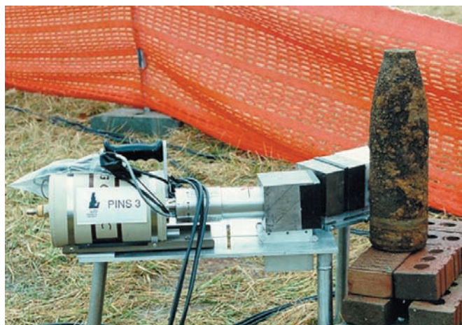
Figure 1. miniPINS inspects an old artillery munition.
