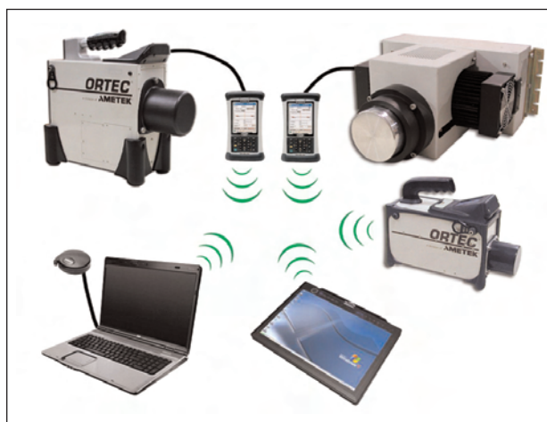
Figure 6. General configuration, multiple detector nodes and separate user interface and analysis computers.
