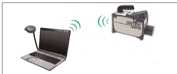
Figure 5. Simplest configuration, one Micro-Detective acts as a single node. Single laptop acts as user interface and analysis computer.
